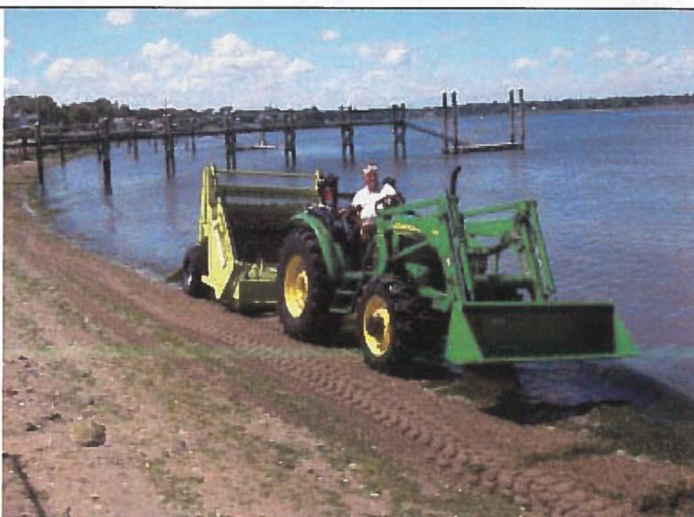
well directly in water as well as wet sand. It can even work in water up to three (3) feet deep. In addition to creating a beautifully manicured beach, the SURF n beach sand. Photo: Door County, WI & RI DEM
