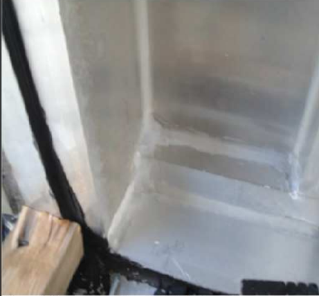
Figure 4: Water leakage through pinhole in caulk at front of chamber
