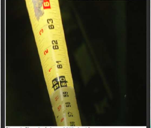
Figure 6: Water depth dropped 1/4" after 1 hour
