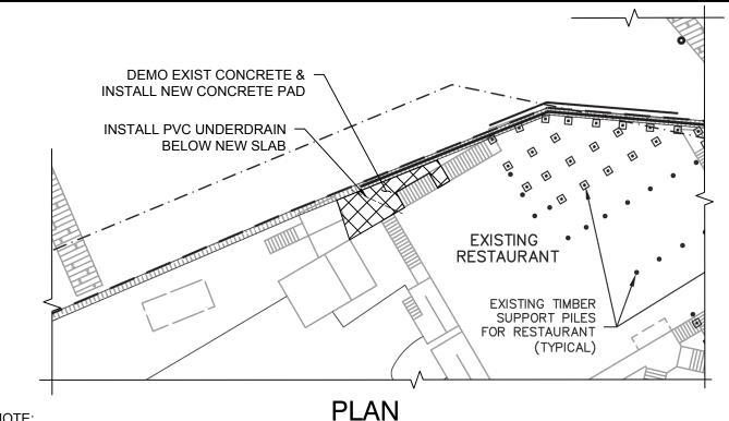
NOTE: SLOPE CONCRETE SURFACE TO DRAIN AWAY FROM RESTAURANT
