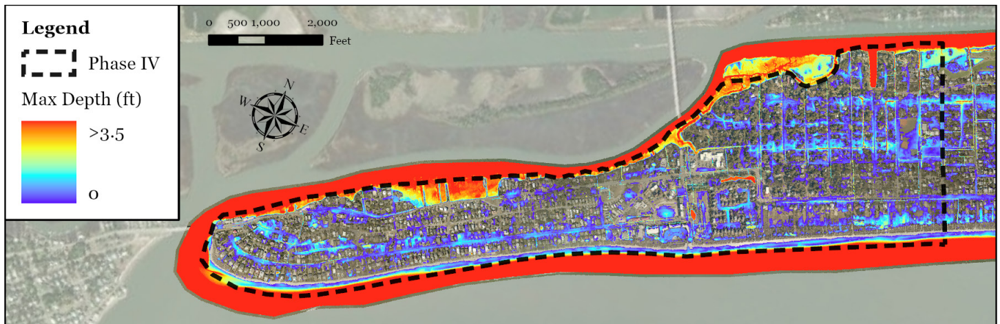
Extents of estimated flooding for Hurricane Joaquin on Isle of Palms (simulated from 2D rain-on-grid model).
