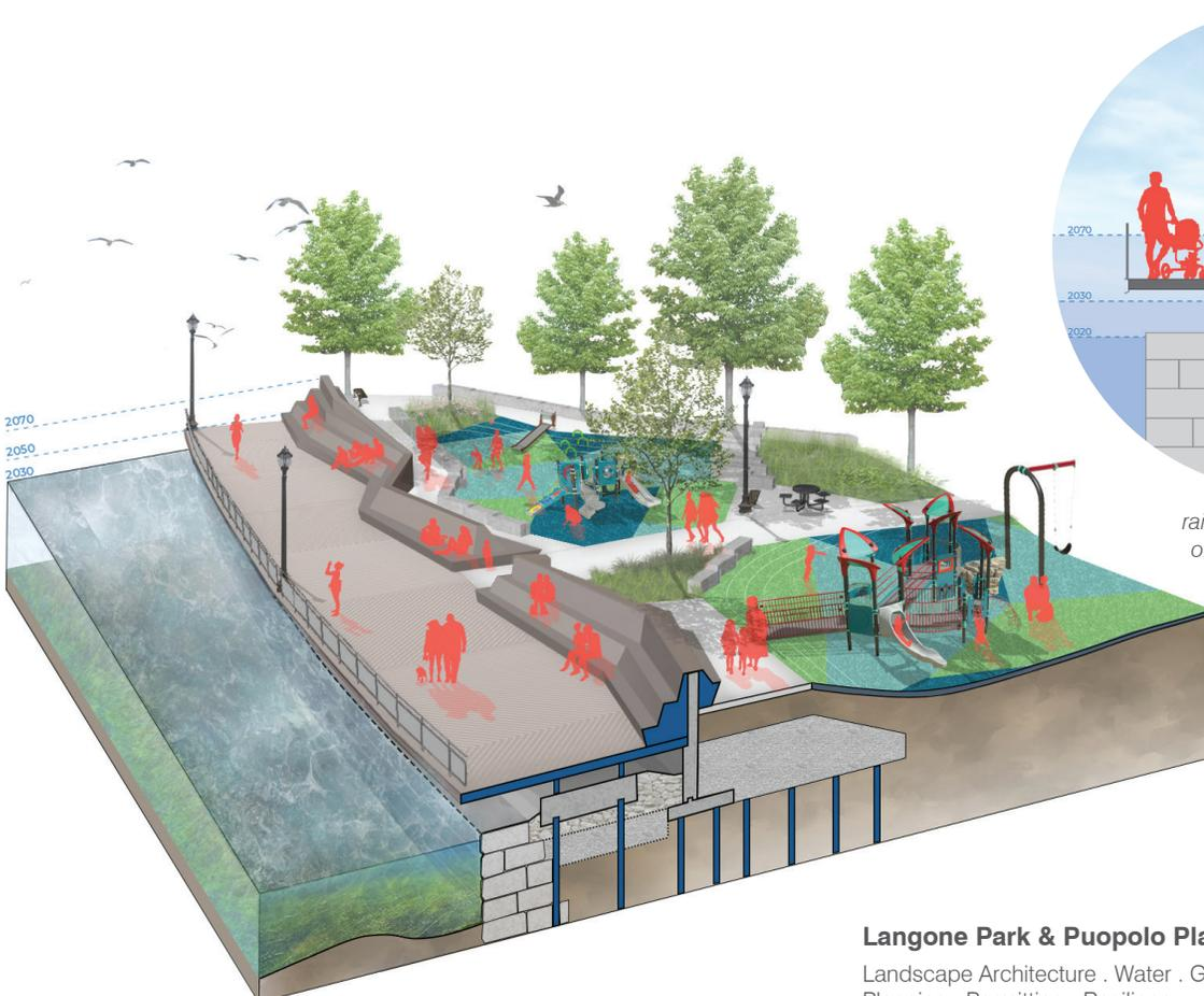
*raised deck built on top of an existing sea wall*
