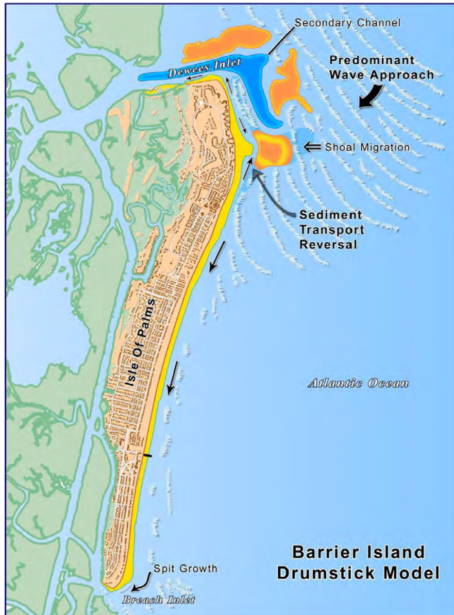
Figure 2. Isle of Palms exhibits a “drumstick” shape due to inlet shoal bypassing at Dewees Inlet at the east end of the island, and westerly sediment transport toward Breach Inlet (bottom). Figure from CSE (2015a).
