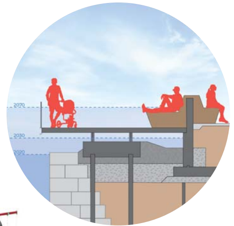
raised deck built on top of an existing sea wall
