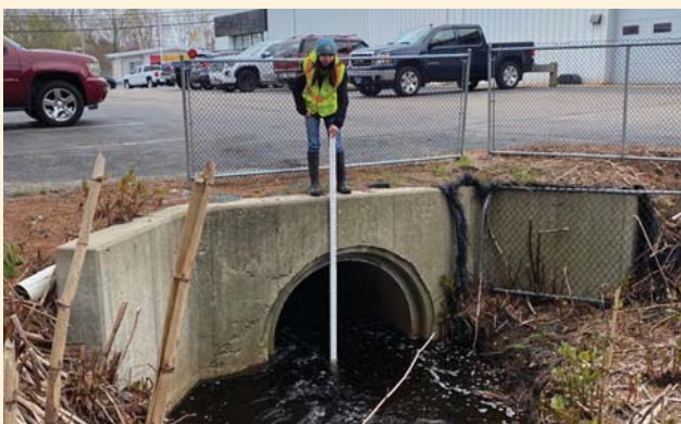
A field team member measuring the diameter of a culvert
