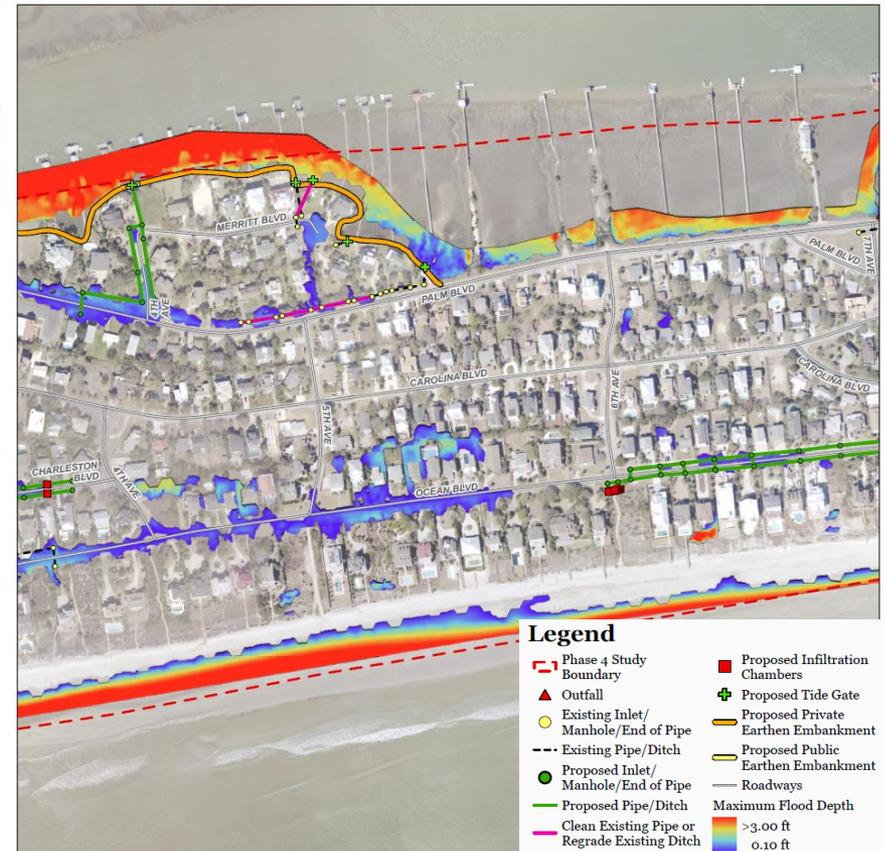
The existing conditions were determined based on the field inventory taken from the survey. The results of a 10-year 24-hour SCS type III (6.60 in) Rainfall with typical tides is shown above for a section of the island on Ocean Blvd and Merrit Blvd.
