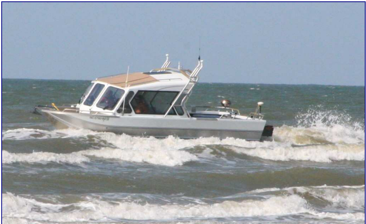
FIGURE 2.2. CSE beach monitoring methods include land-based data collection using Trimble™ RTK GPS from the backshore to low-tide wading depth and over-water work using RTK GPS linked to a precision echosounder aboard CSE's shallow draft boat (RV Congaree River).
