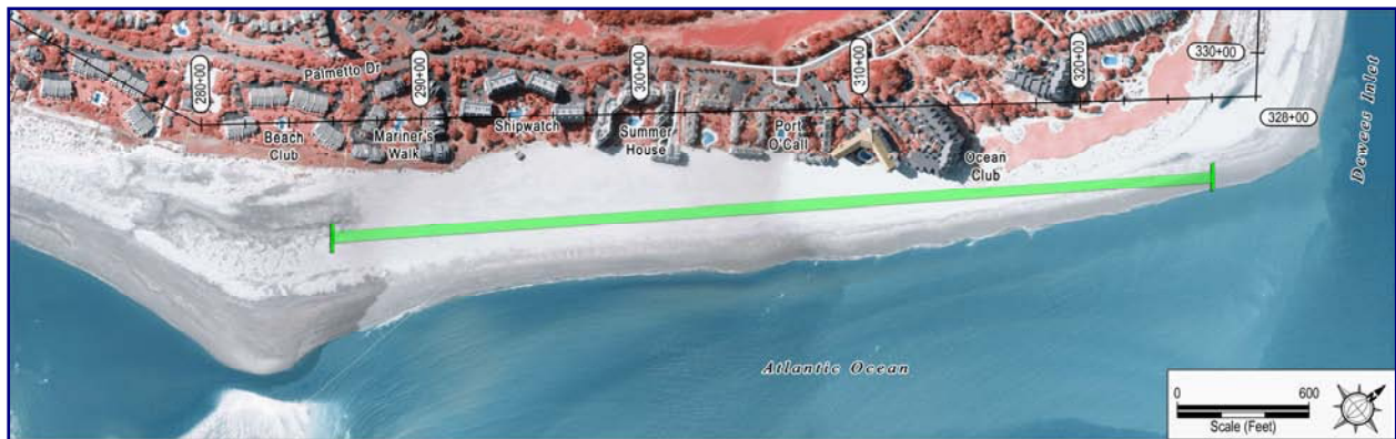
FIGURE 3.9. The North Wild Dunes reach spans from the Wild Dunes Property Owners Beach House (station 280+00) to the 18 th fairway of the Wild Dunes Links Course (station 328+00). The approximate limits of nourishment Reach B are identified by the green bar. March 2009 aerial image by Independent Mapping Consultants Inc.
