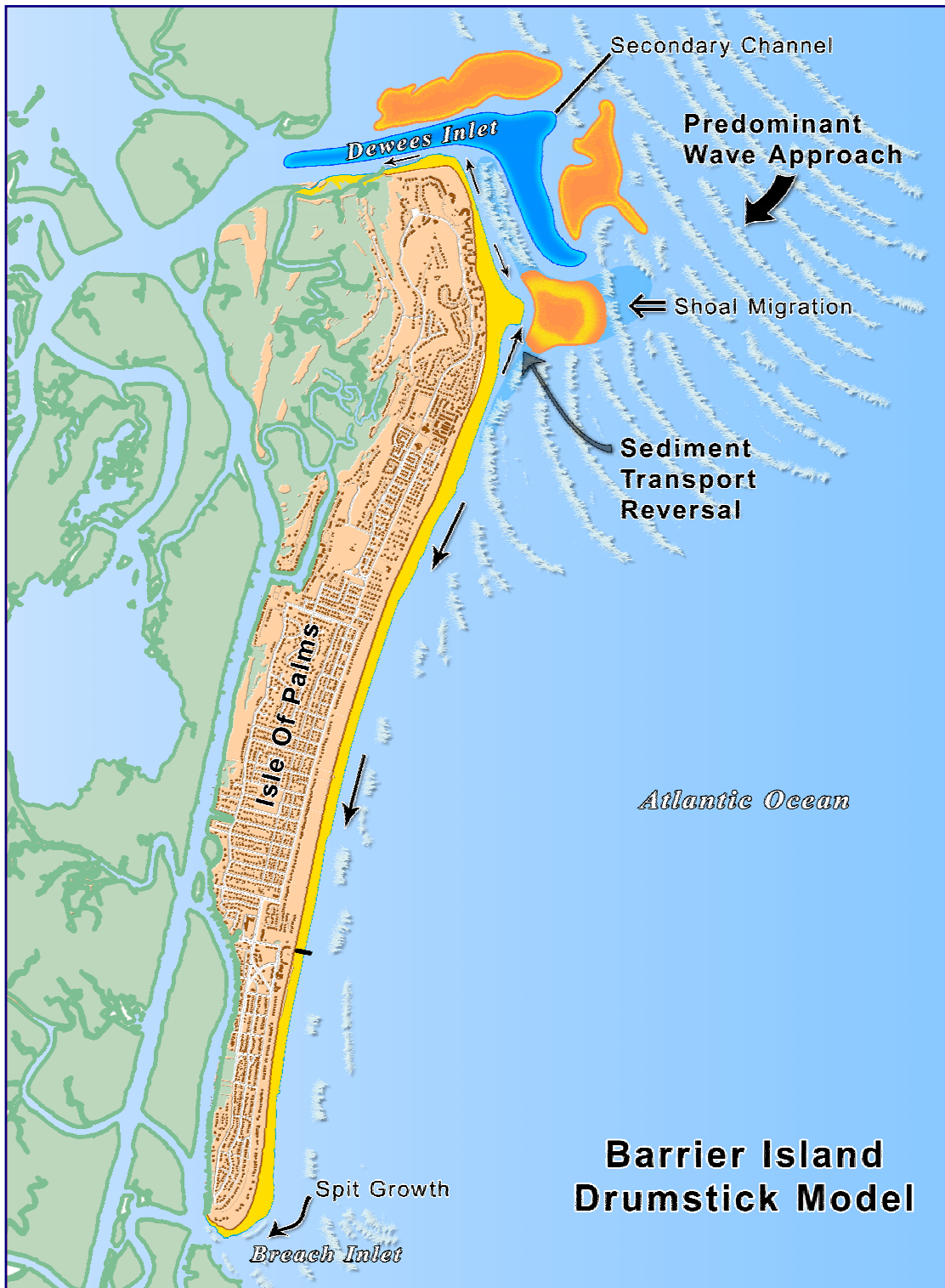
FIGURE 1.2. Isle of Palms is a typical “drumstick” barrier island (after Hayes 1979), where the upcoast end is wider due to sediment accumulation through shoal-bypass events, and the downcoast end usually forms a growing recurve spit. Other examples of drumstick barrier islands along South Carolina are Bull Island, Kiawah Island, and Fripp Island. Zones of sediment transport reversal generally occur in the lee of delta shoals which are situated offshore. Upon shoal attachment to the beach, transport directions in the vicinity of the shoal switch, spreading sand away from the attachment point (cf — Fig 1.4).
