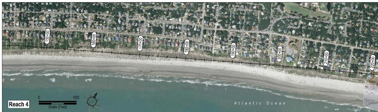
**FIGURE 4.17.** Baseline stationing along Reach 4 spanning the length of beach between 31<sup>st</sup> Ave and 53<sup>rd</sup> Ave.
