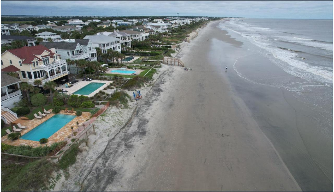
**FIGURE 4.26.** Aerial view of Reach 2 in September 2024. Since monitoring began in 2009, Reach 2 has been the most stable reach, typically showing lower magnitudes of volume change compared to the other reaches along Isle of Palms. The arc in the shoreline west of the pier indicates that the pier may act to trap sand, which may impact Reach 2 in certain wave conditions.
