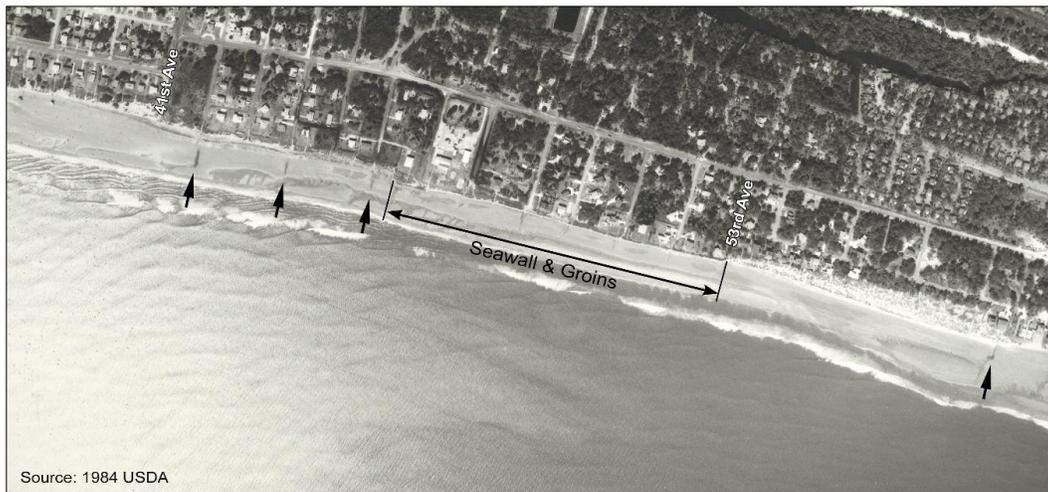
**FIGURE 2.4.** A seawall and groins were in place in 1984 between 46<sup>th</sup> Ave to 53<sup>rd</sup> Ave. Today, due to rapid accretion, these groins and seawalls have been buried.
