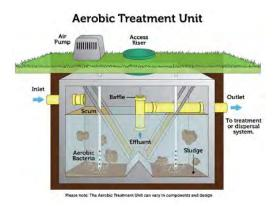
Figure 6-3. Advanced (Aerobic)
