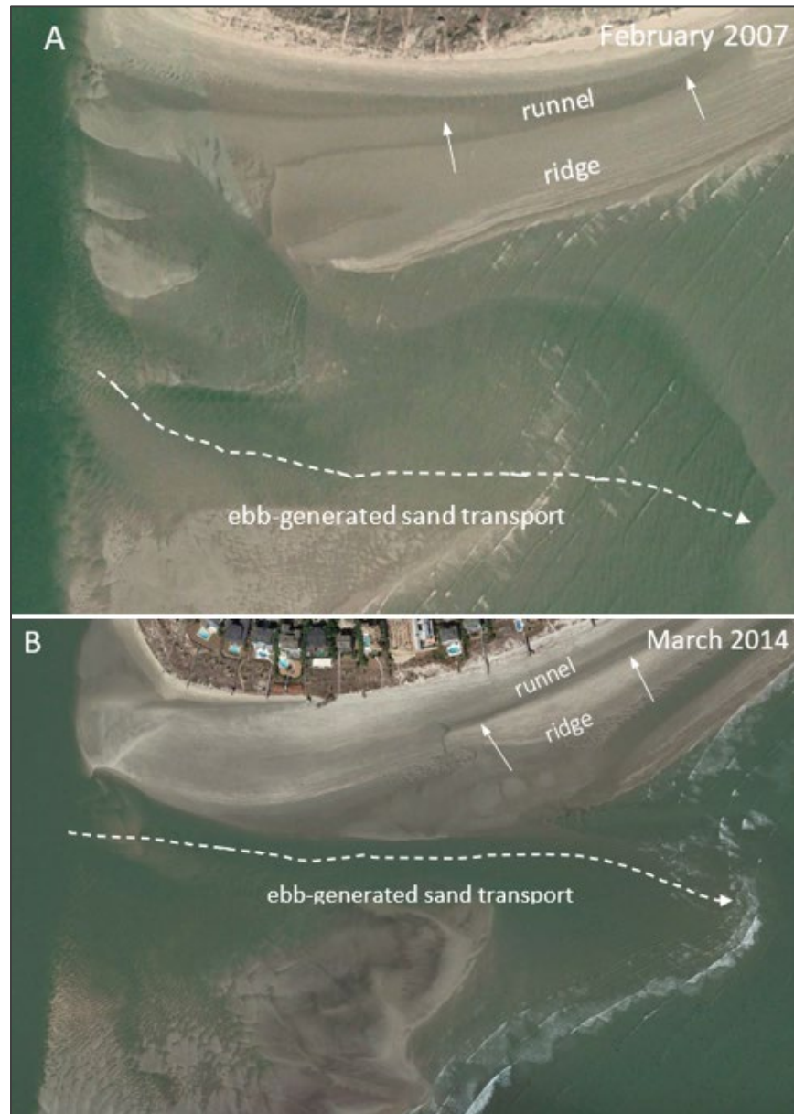
Figure 13. Ebb-spillover lobes at Breach Inlet in 2007 (A) and 2014 (B), showing sand transport pathways and the formation of ridge and runnel systems along the beach.
