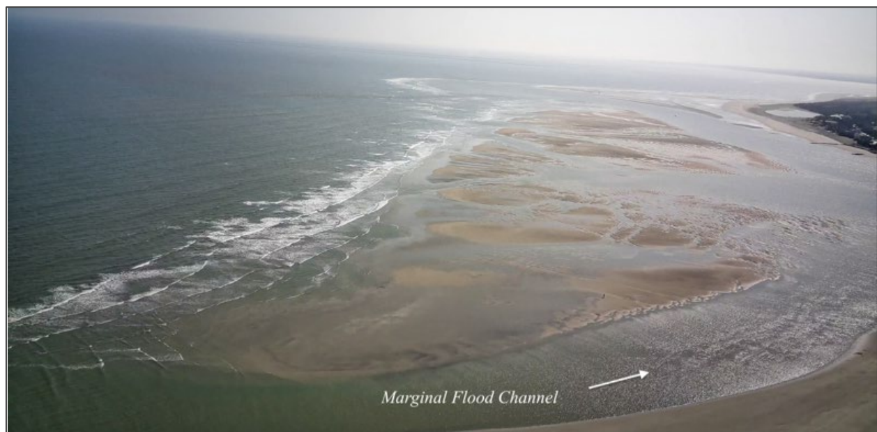
Figure 8. Recent photograph (03/2025) of the nearshore zone at the southern end of the Isle of Palms, showing a well-developed marginal flood channel. The channel enhances wave-driven sediment transport toward Breach Inlet.
