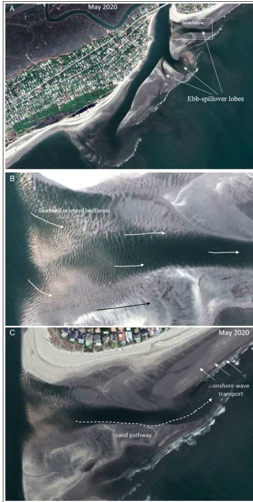
Figure 12. Sand transport seaward through ebb-spillover lobe. A: Inset identifying ebb lobe close to beach. B: Inset showing ebb-oriented bedforms indicating seaward transport to the east. C: Image demonstrating that seaward transport of sand moves onshore by wave action.
