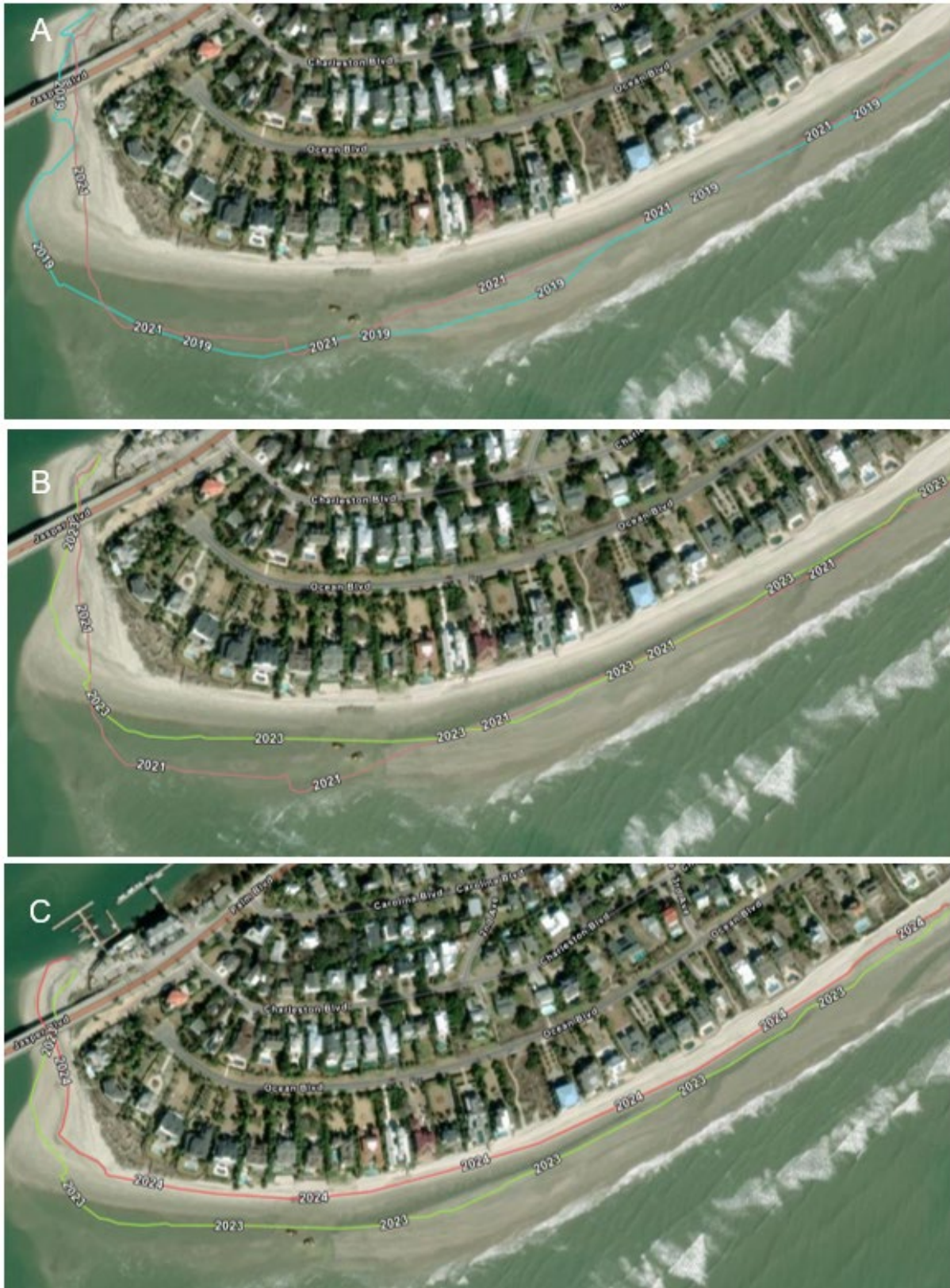
Figure 5. Shoreline changes near Breach Inlet. A. 2019 and 2021, B. 2021 and 2023, C. 2023 and 2024. Note the gradual retreat of the shoreline from 2019 to 2024.
