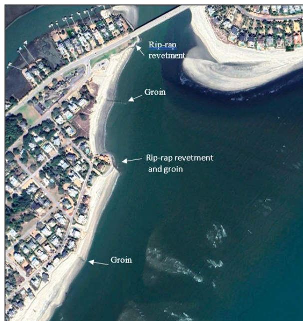
Figure 3. Recent (03/2025) aerial photo of Breach Inlet and the northwest end of Sullivan's Island. The structures identified in the image have served to stabilize the inlet's location and reduce erosion.
