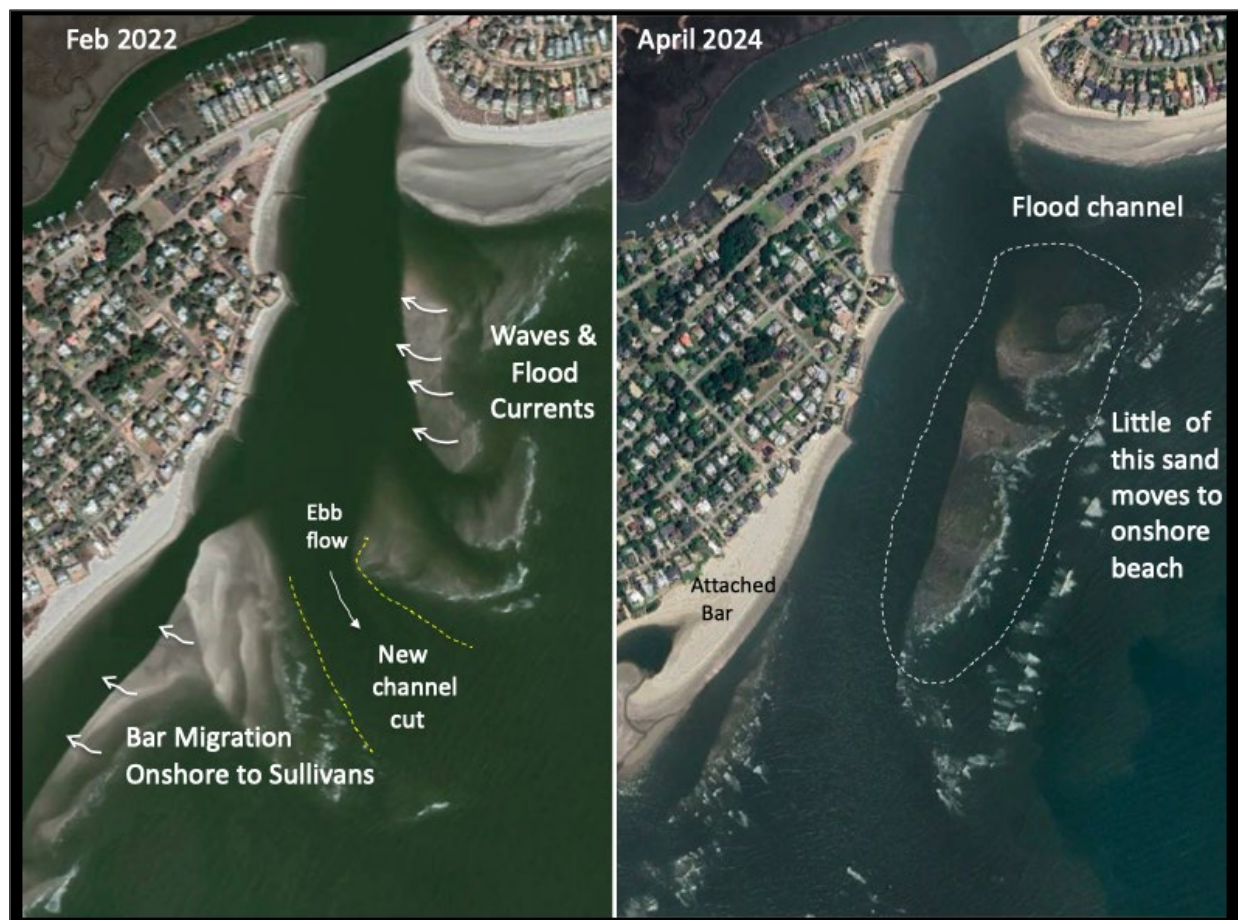
Figure 11. Photographs of the ebb-tidal delta from 2022 and 2024, showing the formation of a new channel across the distal delta in 2022, which facilitated sand bypassing Breach Inlet and led to a bar welding onto Sullivan's Island.
