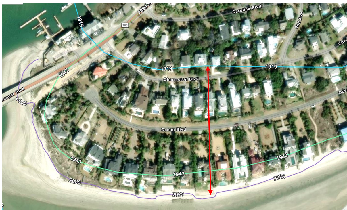
Figure 4. Aerial photo of the southwestern end of Isle of Palms showing the position of the highwater shoreline in 1919, 1943, & 2025. During this +100-yr period the ocean shoreline built seaward by almost 200 m (see red arrow).
