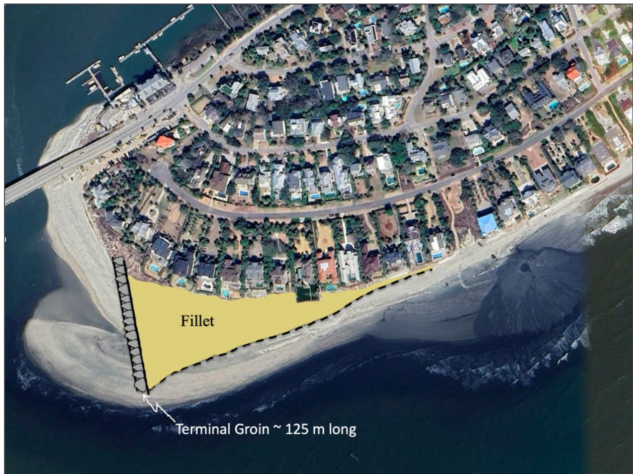
Figure 15. Concept sketch of a terminal groin and associated beach fillet illustrating this concept for the southern end of Isle of Palms adjacent to Breach Inlet.
