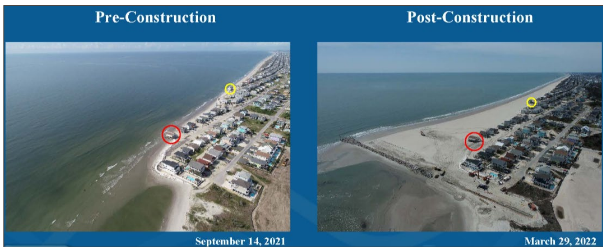
Figure 17. Before/after photos of the terminal groin at Ocean Isle Beach, Brunswick County, NC.
