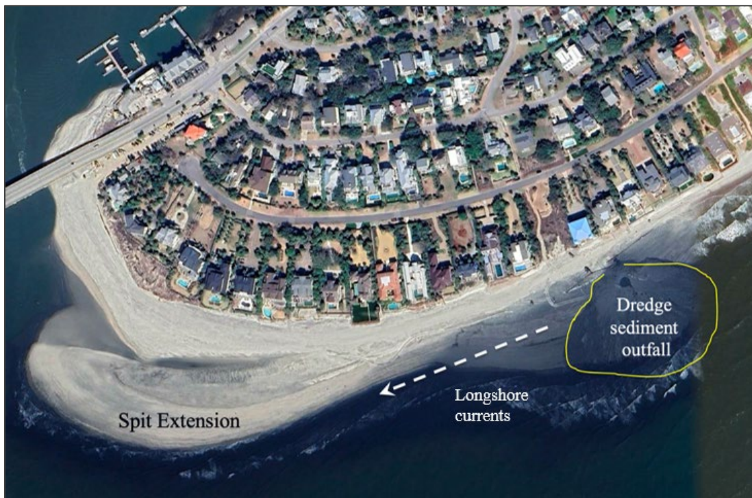
Figure 10. Recent aerial photograph (03/2025) showing the dredging operation and the formation of a sand spit driven by longshore sediment transport.
