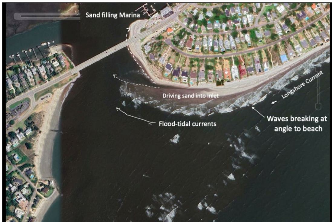
Figure 9. Aerial photo from 04/2024 showing angular wave approach generating southerly longshore currents, which are further enhanced by flood-tidal currents entering Breach Inlet.
