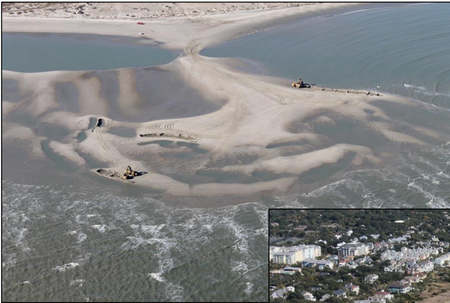
Figure 1. Photos from the 2014-2015 shoal management project showing sand harvesting from the attaching shoal and from a harvest area just north of 53rd Ave.
