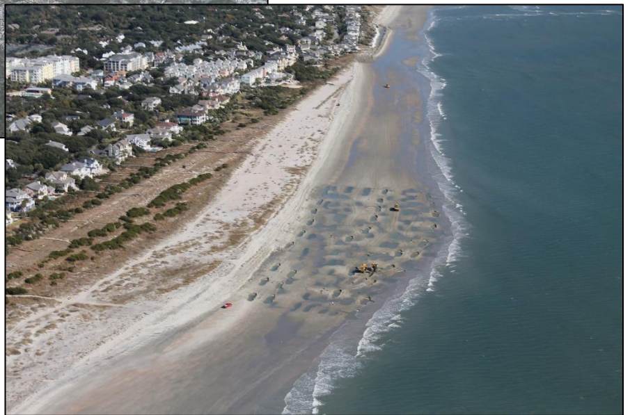
Figure 1. Photos from the 2014-2015 shoal management project showing sand harvesting from the attaching shoal and from a harvest area just north of 53rd Ave.
