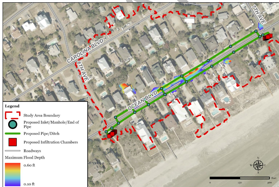
b) Proposed Drainage Improvements
