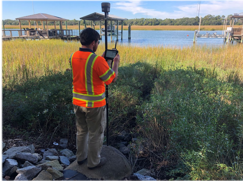
Figure 3 – Example of drainage system inventory using GPS units at an outfall along the intracoastal waterway.
