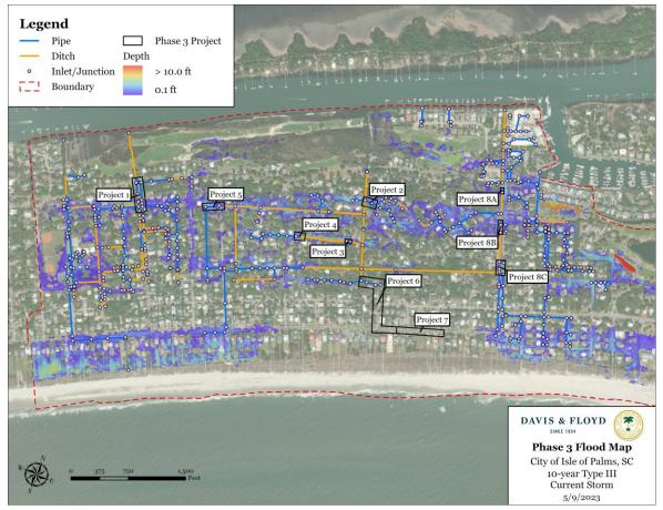
The existing conditions were determined based information provided by the town. The results of a 10-year 24-hour SCS type III (6.60 in) Rainfall is shown above for the Phase 3.
