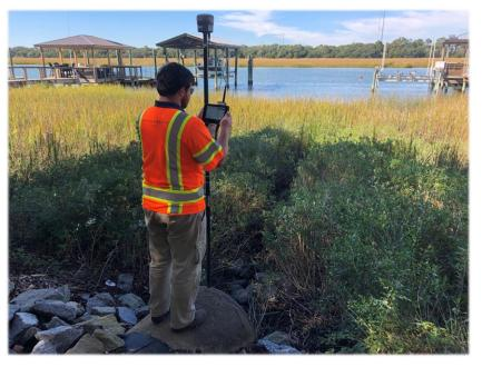
Example of surveying the drainage system inventory using the GPS units. This photo was taken at an outfall going to the intracoastal waterway.
