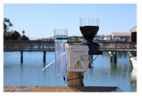
Example of a monitoring system placed on the island to monitor the rainfall and tidal conditions. This monitor was placed at the marina along the intracoastal waterway.
