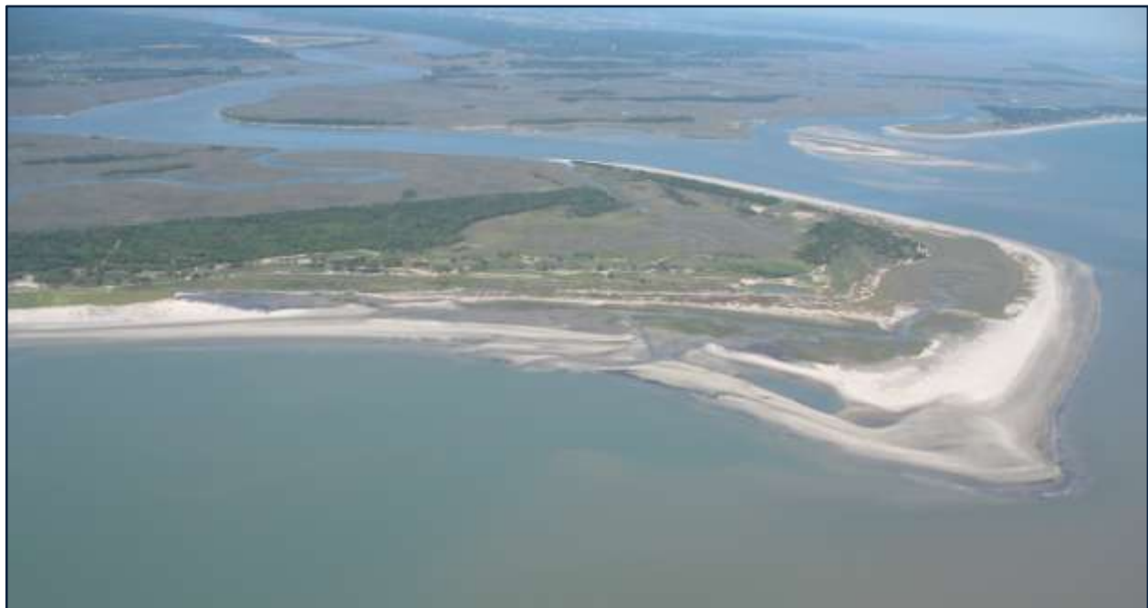
FIGURE 3.40. Shoal-bypass events at Kiawah Island. The upper image from 1998 shows two shoals estimated to contain ~5 million cubic yards of sand. Shoal 1 was attached and had built a barrier beach ~1,500 ft seaward of the original shoreline. A marsh was forming in the created lagoon. The second shoal was attached at the north end, but still in Stage 2 of the bypass cycle at the south end. The lower image is the same area in April 2010. By this time the second shoal had completely attached and was in the process of forming a new outer beach. Marsh had developed throughout the lagoon, leaving a network of tidal creeks flushing the new system. [Source: CSE 2007, 2010]
