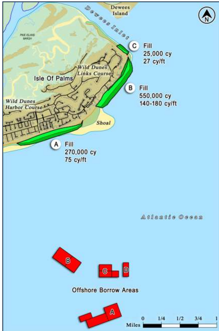
FIGURE 1.4. Project map of the 2008 IOP restoration project. The project was designed to nourish sections of the beach and provide sufficient sand to offset losses associated with long-term erosion as well as an ongoing shoal-bypass event. Borrow areas were located 2-3 miles offshore. Area D was not dredged.
