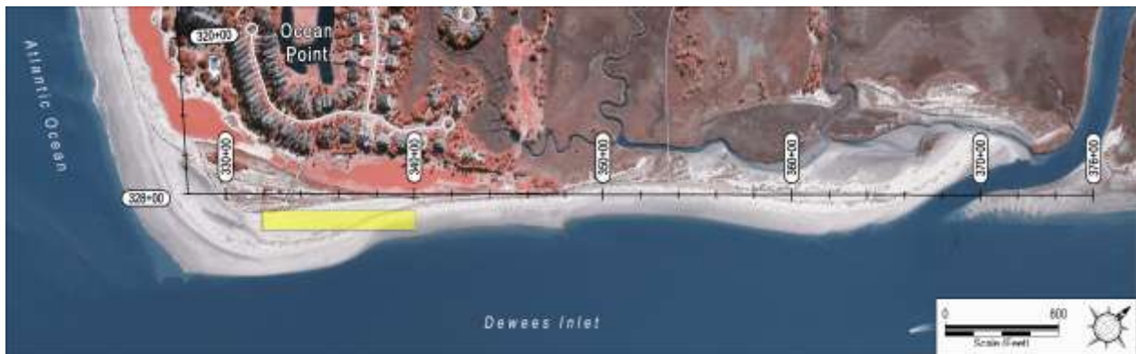
FIGURE 3.3. Station map of the Dewees Inlet area (Reach 7). Reach 7 spans from station 330+00 near the 18 th tee to station 368+00 near Cedar Creek spit. The approximate limits of nourishment Reach C are identified by the yellow bar. The 1981 low profile groin is positioned near station 348+00. [March 2009 aerial image by Independent Mapping Consultants Inc]
