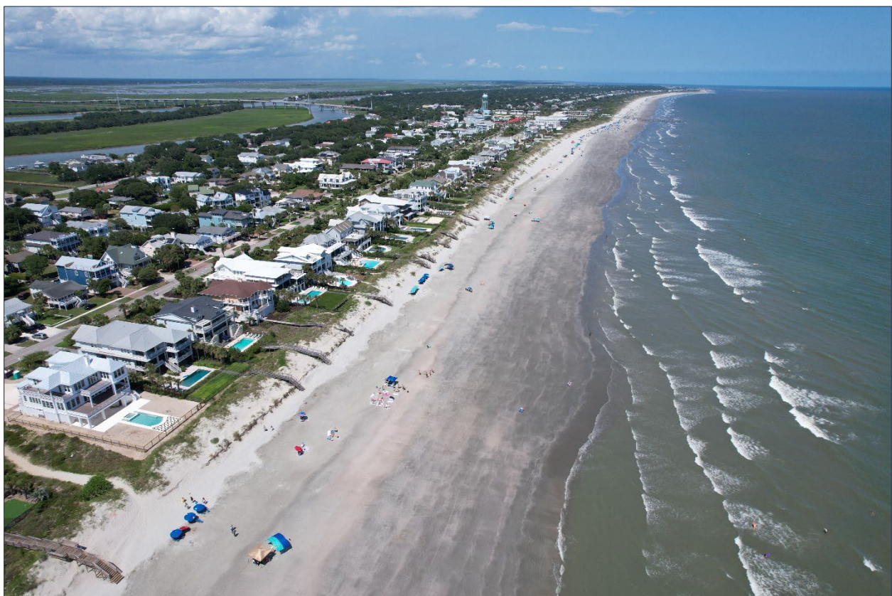
FIGURE 4.26. Aerial views of Reach 2 in Aug 2023. Since monitoring began in 2009, Reach 2 has been the most stable reach, typically showing lower magnitudes of volume change compared to the other reaches along Isle of Palms. The arc in the shoreline west of the pier indicates that the pier may act to trap sand, which may impact Reach 2 in certain wave conditions. Erosion over the past year has reduced the beach width, especially south of 7 th Ave.
